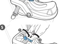
4 While holding taut, slide shoulder belt back through the belt path as close as possible to the top of the lock-off. **NOTE:** Tightness indicator should be **GREEN**.
